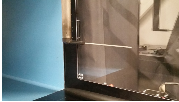
Figure 3.6: Photograph of the downstream CTA hotwire (hW3) installed in the wind tunnel test section.
