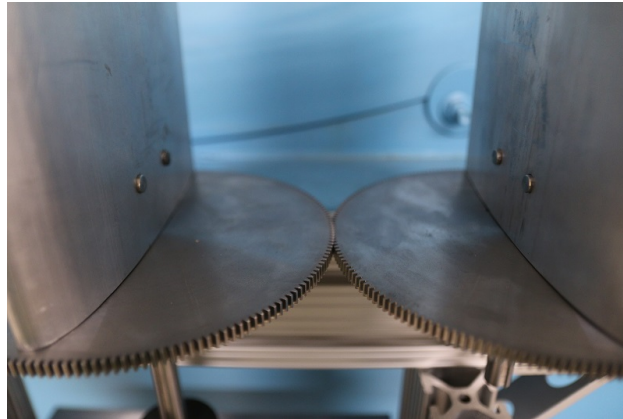
Figure 3.3: Close-up of the gust generator gears and airfoil vane connection.
