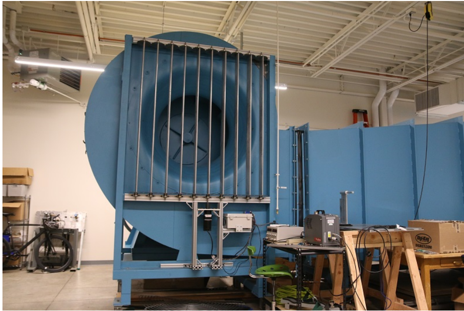
Figure 3.1: Gust generator system installed on the inlet of the CU Boulder low-speed research wind tunnel.
