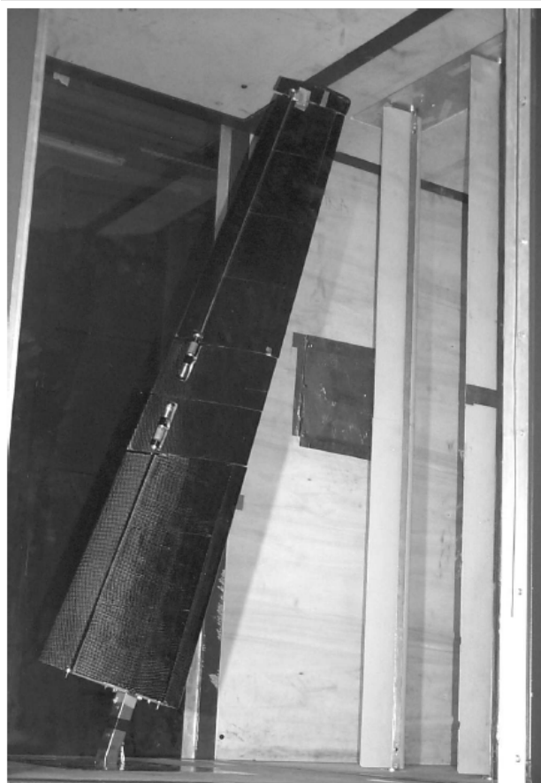
Figure 1.3: The Unsteady facility at Politecnico di Milano. The pair of gust generation vanes are seen to the right of the airfoil being tested[18].
